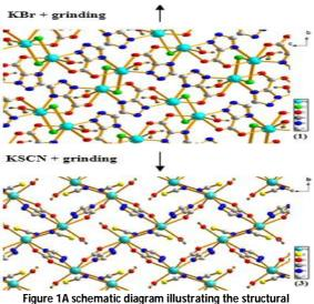
conversions from 3D coordination polymer 1 (middle) to 3D coordination polymers 2 (up) and 3 (bottom) by solid state irreversible anion-replacement.
