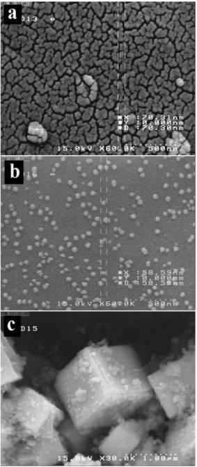
Figure 2The SEM images of (a) PbCl<sub>2</sub>, (b) PbBr<sub>2</sub> and (c) cubicshaped PbS nanoparticles prepared by thermolysis of compounds 1, 2 and 3 in oleic acid at 200 °C under air atmosphere for 2 h, respectively
