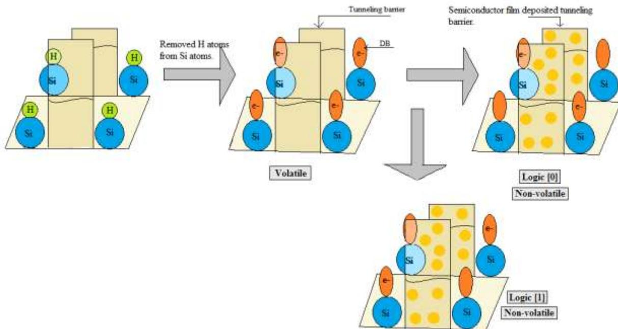
**Figure 3** | Proposed architecture for the non-volatile quantum dot cellular automata based device.
