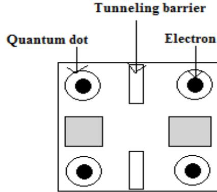
**Figure 1** | Typical view of the QCA cell.
