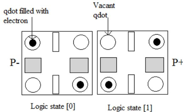
**Figure 2** | States of the logic for QCA
