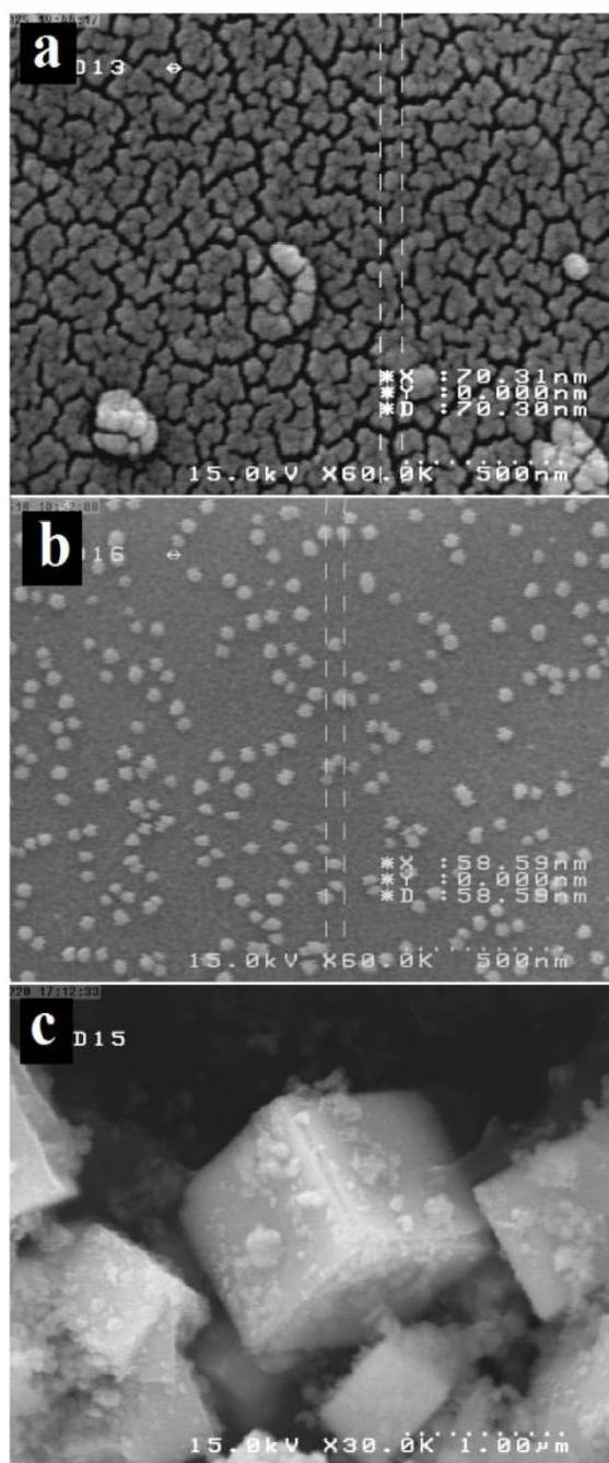
Figure 2 The SEM images of (a)  $\text{PbCl}_2$ , (b)  $\text{PbBr}_2$  and (c) cubic-shaped  $\text{PbS}$  nanoparticles prepared by thermolysis of compounds 1, 2 and 3 in oleic acid at 200 °C under air atmosphere for 2 h, respectively
