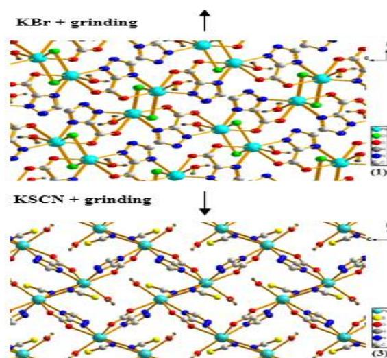
Figure 1A schematic diagram illustrating the structural conversions from 3D coordination polymer 1 (middle) to 3D coordination polymers 2 (up) and 3 (bottom) by solid state irreversible anion-replacement.
